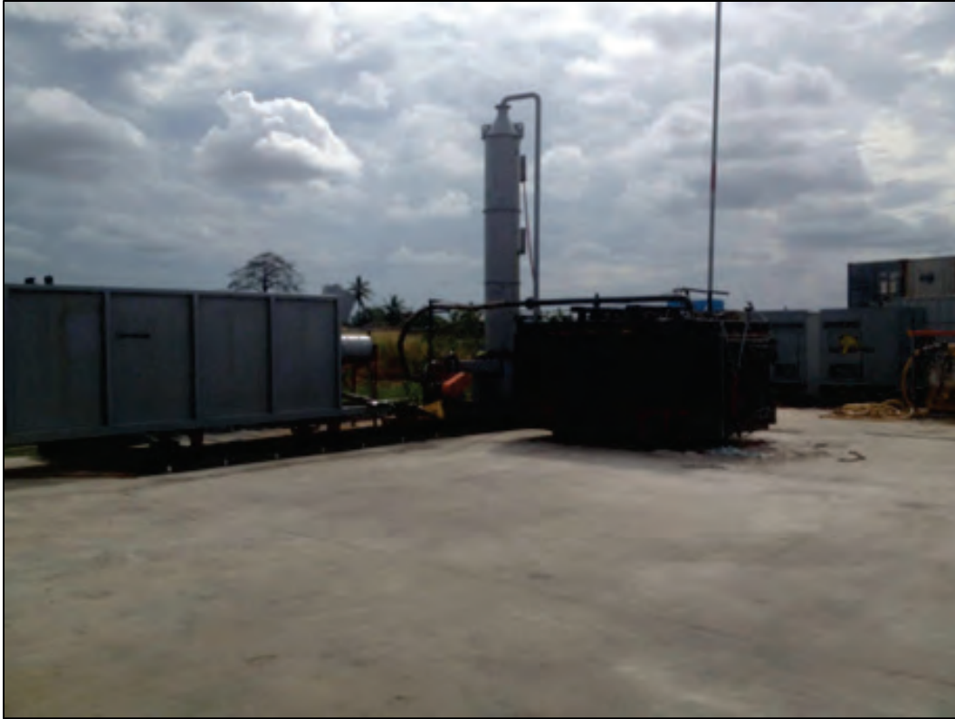
Figure 2.10-6: Vertical Infrared Unit with Wet Scrubber and Oxidizer at Typical Waste Management Facilities
