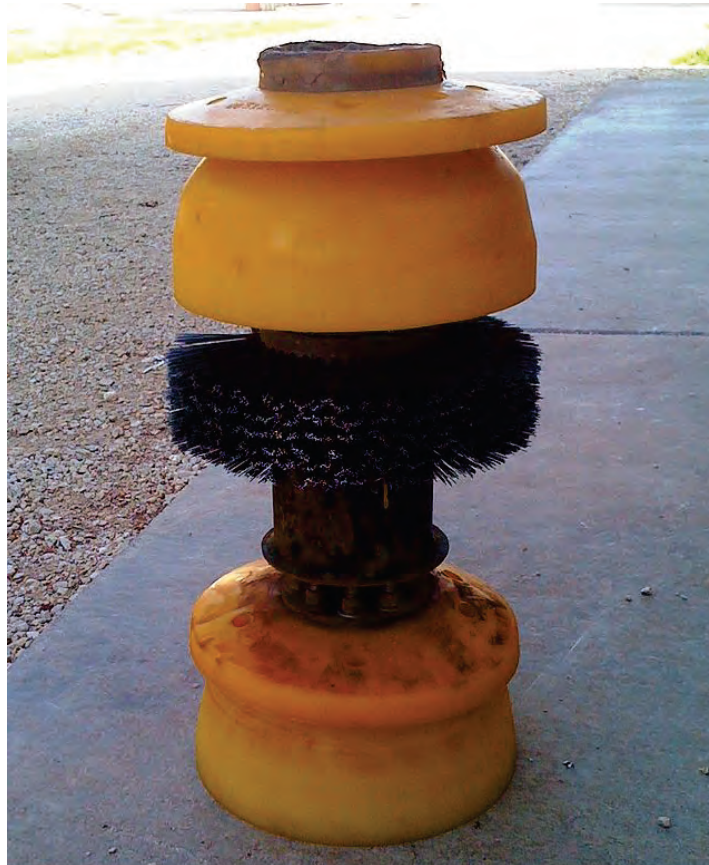
Figure 2.6-2: Example of Wire Brush Cleaning Pig
